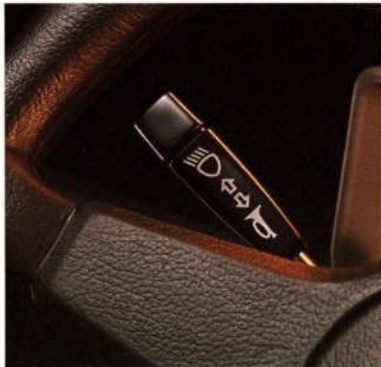
Twin column stalk controls give quick and easy access to indicators, horn, headlamp dip/flash (left) and wipers and washers (right).
