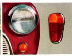
12 volt headlamps with dipper and separate flashers. Tail-lamp assemblies house rear lights, reflectors and flashers, separately, in one unit.
