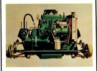
more room inside. Engine, clutch, gears, differential, and transmission take up only 18 inches of the car's length. And there's a new short, sporty, remote-control gear lever. If preferred however, the Super De-luxe Saloon is also available with the optional 848-c.c. engine and direct control gear-change. Servicing of this remarkable power unit is quick and
