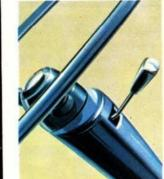
A single switch on the steeringcolumn incorporates dip switch, headlamp flasher, horn, and selfcancelling direction indicators; thus providing a single source of all communications with other road users.
