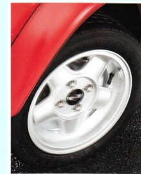
REVOLUTION ALLOY WHEEL (5 SPOKE) WHEEL DIMENSION 6J X 13"
