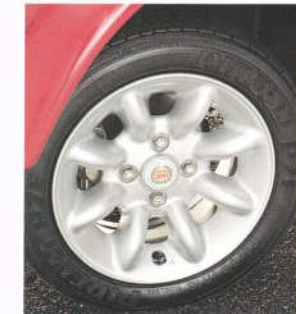
SPORTS ALLOY WHEEL (8 SPOKE) WHEEL DIMENSION 6J X 13"
