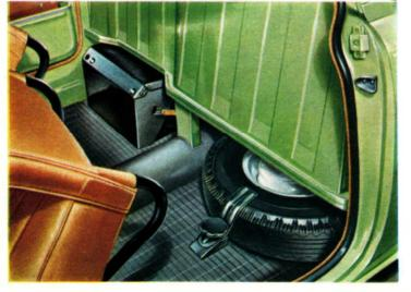
Another example of the great attention paid to detail, which helps to reduce routine service time spent on the 1-ton commercials—the driver's seat (and passenger's seat, when fitted) hinges forward to permit access to the battery, and to the spare wheel, which is securely held by a quick-release metal strap. Being positioned beneath the actual floor level, they are instantly available whether the vehicle is loaded or not.
